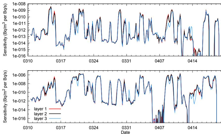
**Fig. 3.** Sensitivity of the station network to  $^{137}\text{Cs}$  emissions at FD-NPP, for the atmospheric concentration measurements (upper panel) and for the deposition measurements (lower panel). The sensitivities are calculated separately for emissions at the lowest layer (0–50 m, red), middle layer (50–300 m, black) and top layer (300–1000 m, blue).
