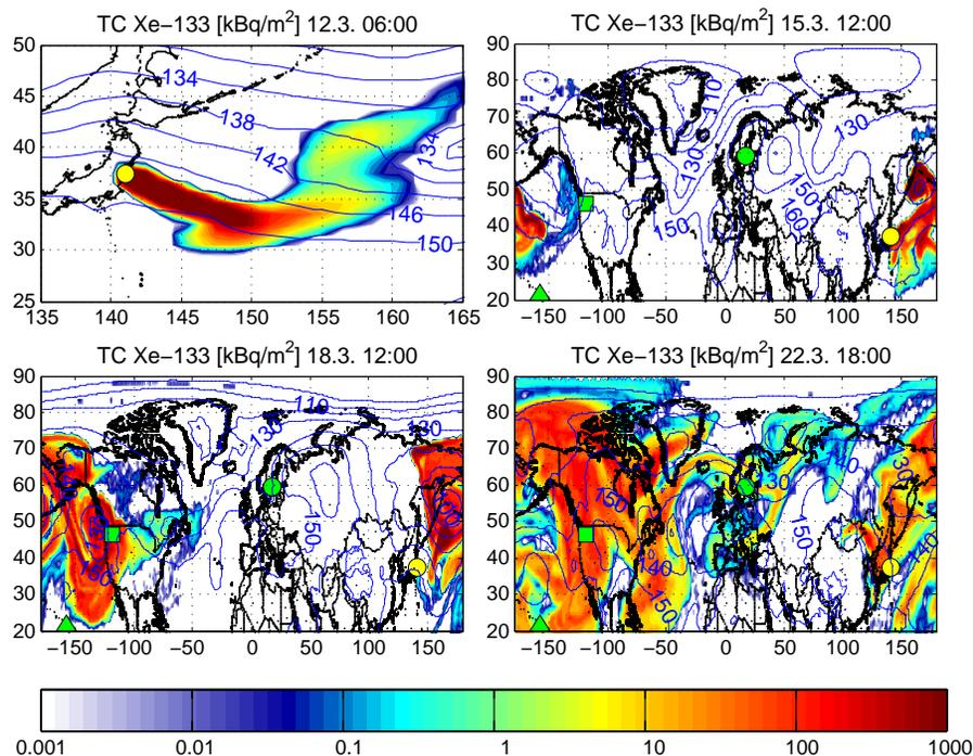
**Fig. 13.** Simulated total atmospheric columns of  $^{133}\text{Xe}$  (color shading) and geopotential at 850 hPa from GFS (blue isolines) at 06:00 UTC on 12 March (upper left panel), 12:00 UTC on 15 March (upper right panel), 12:00 UTC on 18 March, and 18:00 UTC on 22 March. The location of FD-NPP is shown with a yellow circle, the station on Oahu (Hawaii) with a green triangle, Richland (USA) with a green square, and Stockholm (Sweden) with a green circle.
