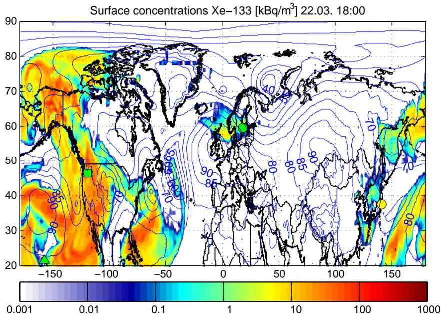
**Fig. 18.** Surface concentrations of  $^{133}\text{Xe}$  (color shading) and geopotential at 925 hPa (blue iso-lines) at 18:00 UTC on 22 March. In the lower panel, the stations Oahu (Hawaii) and Stockholm (Sweden) are marked with a green triangle and a green circle, respectively.
