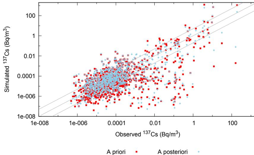
**Fig. 9.** Scatter plot of observed and simulated <sup>137</sup>Cs concentrations, based on a priori (red squares) and a posteriori (blue crosses) emissions. The gray line in the middle is the 1:1 line and upper and lower lines represent factor of 5 over- and underestimates.
