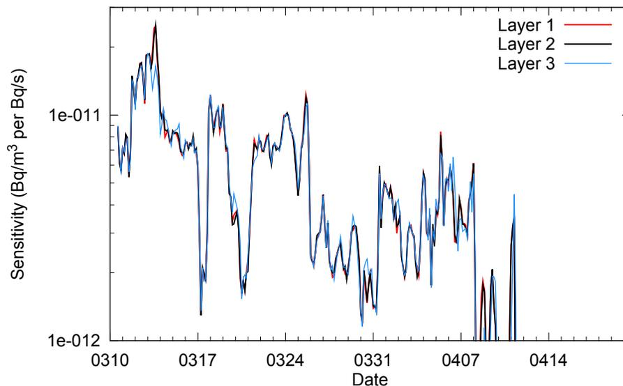
**Fig. 2.** Sensitivity of the station network to  $^{133}\text{Xe}$  emissions at FD-NPP. The sensitivities are calculated separately for emissions at the lowest layer (0–50 m, red), middle layer (50–300 m, black) and top layer (300–1000 m, blue).
