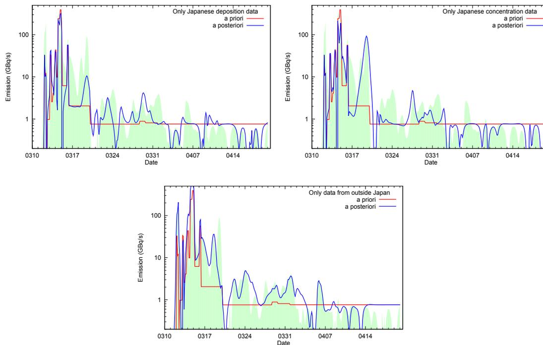
**Fig. 6.** Sensitivity of  $^{137}\text{Cs}$  a posteriori emissions to changes in the input measurement data: when using only Japanese deposition data (top left panel), when using only Japanese concentration data (top right panel), and when using only non-Japanese concentration data (bottom panel). Shown are a priori emissions (red line), a posteriori emissions (blue line) and a posteriori emissions based on the full data set (repeated from Fig. 5, green shading in background).
