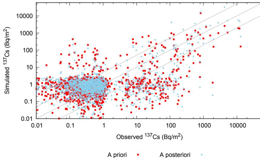
**Fig. 11.** Scatter plot of observed and simulated  $^{137}\text{Cs}$  deposition values, based on a priori (red squares) and a posteriori (blue crosses) emissions. The gray line in the middle is the 1:1 line and upper and lower lines represent factor of 5 over- and underestimates.
